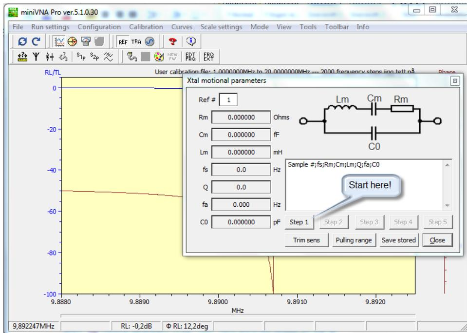
The 5 buttons marked "Step 1" to "Step 5" do the necessary measurements and calculations. Please give the unit time to make sweeps – a progress bar in main window, just above the status line, shows the progress of the sweep.
