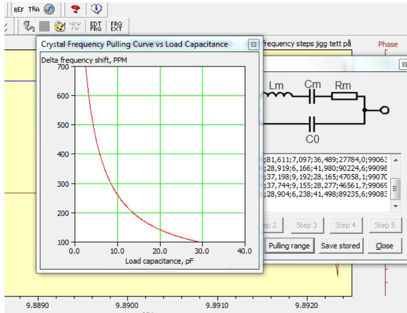
The “pulling curve” is only shown for the last Xtal examined. The window is sizable and by right click in the graphical area, the graph could be copied to the clipboard to be transferred to other programs.
