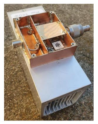
Two 100Ohms power resistors i parallell makes the dummy load, capable of disipating about 300W. The box is splitted in two parts, and the «attenuator» is in the biggest one and just a 30mm rigid cable in the other part – this to get more isolation.
