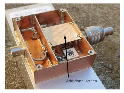
I hope this is enough information to a copy of mine. I mostly use it on HF and sometimes on 2m, and it works for me. The small resitors on output and as the shunt are of MRS 16000 S type. They are 0.4W professional thin film resistors. 15x15ohms and 2x100ohms in addition to the prower resistors.
